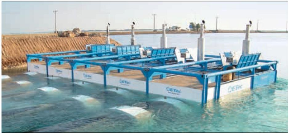
Founded by Eric Thiriez in Cartagena, Colombia, ETEC's initial goal was to build stationary flow pumps for government companies. Because, in some locations, the shore would be too soft for the weight of the stationary pumps, ETEC had to find an alternative to heavy construction. A pump floating in water was the solution.
