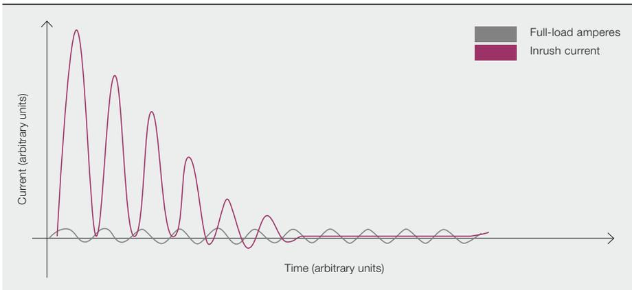
the transfer so the flux does not exceed the saturation point of the transformer's core. Energizing a transformer results in a potential peak inrush current of 5 to 12 times full-load ampacity (FLA); transferring between out-of-phase sources results in a peak inrush current of up to 20 times FLA → 7.
