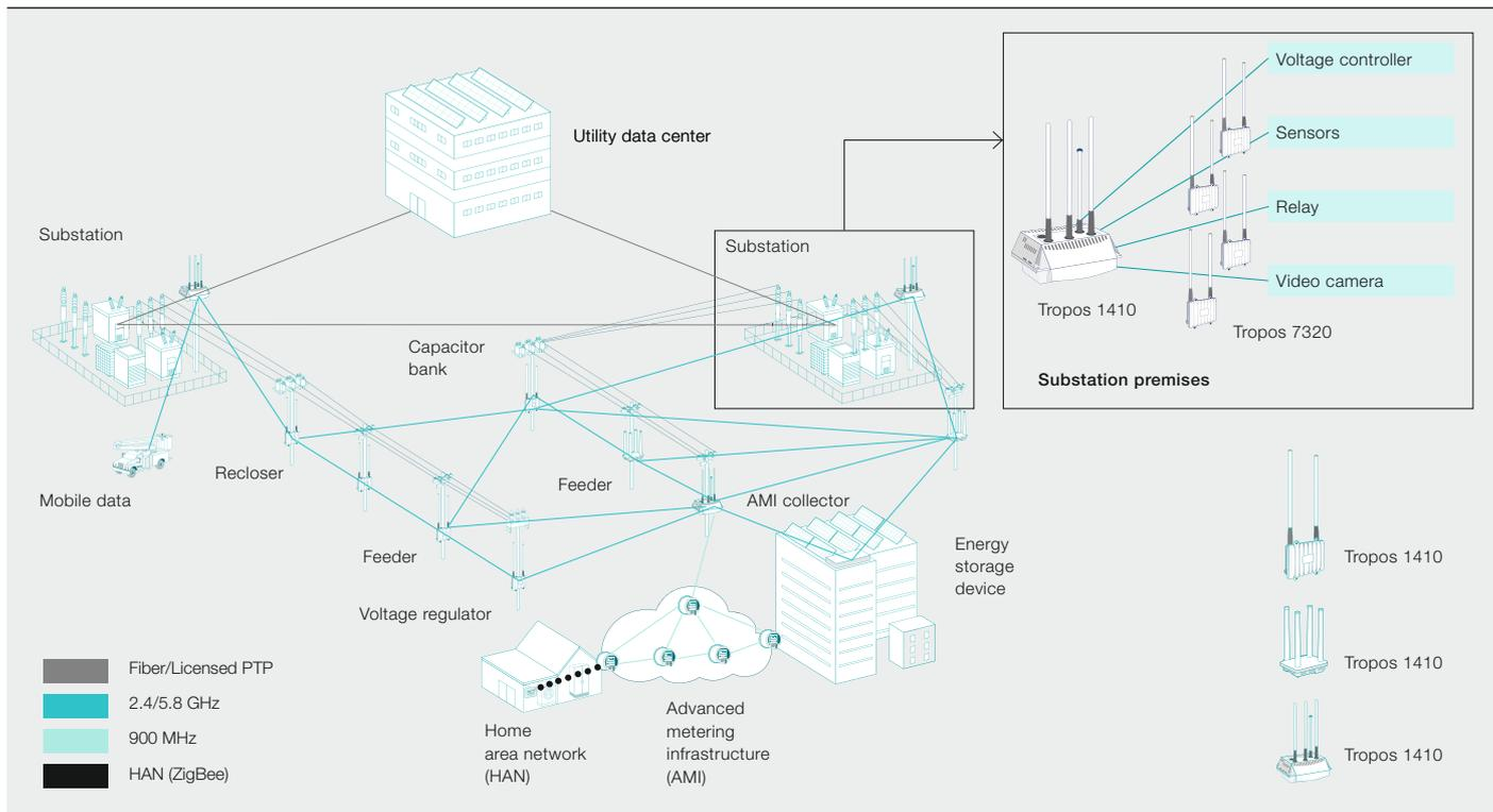
The distributed Tropos mesh architecture is capable of quickly and seamlessly routing around interference and congestion bottlenecks.
